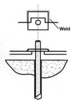
Threaded bar cast in threaded sleeve, hexagon headed bolt used as hold down bolt
