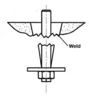
Notched soleplate, cover plate then site drill holding down bolt holes
